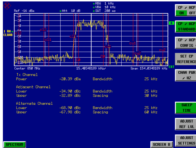
Fig. 2-39 Measuring the relative adjacent channel power of an NADC signal in each of the two adjacent channels below and above the transmit channel.
